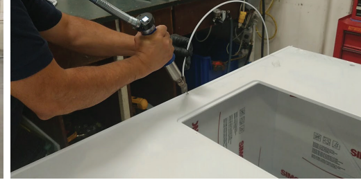
From left to right: SIMONA FM 4910 sheet being welded; Wafab pre-cutting material for fabrication; Close-up of FM 4910 sheet being edge welded
